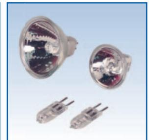
**Bulbs** supplied are 12V/50W/75W halogen. Optional 12V/50W/75W Dichroic Lamps dissipate 60% of heat through back of lamp thus reducing the amount of heat projected forward.
