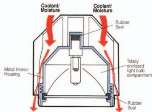
**Moisture-proof lens/reflector/lamp compartment** is totally enclosed by a metal interior housing and rubber seals making the lamps ideal for even the harshest applications.
